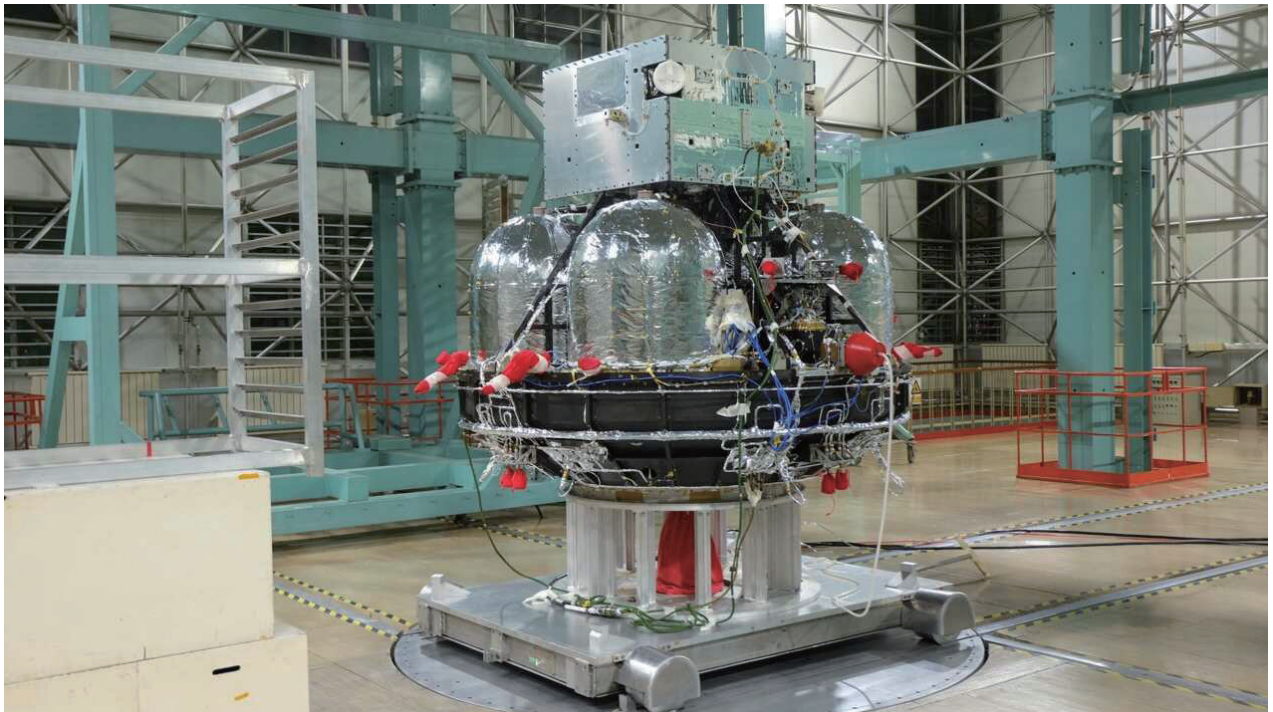
Fig. 5. Magnetic testing of the SMILE flight model.
